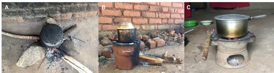
Figure 2 (A) Three stone fire, (B) firewood cookstove—'chitetezo mbaula', (C) charcoal cookstove.
