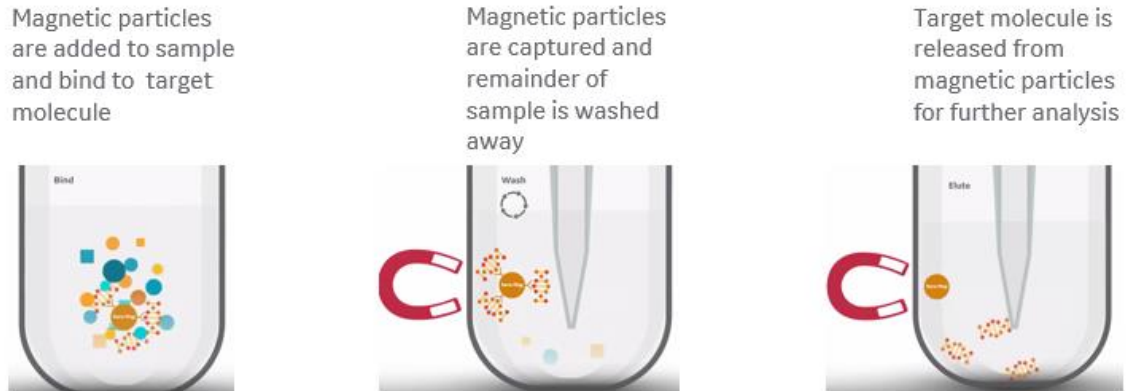
Figure 19 DNA extraction using magnetic particles. Source: Cytiva Life Sciences
