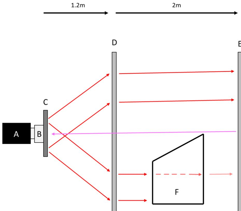
Figure 11. Set-up of room scale tracking recording system. Adapted from (Voloshin et al., 2020). (A) camera, (B) lens, (C) LED ring light, (D) Fresnel lens, (E) Retroreflective screen, (F) bednet and volunteer.
