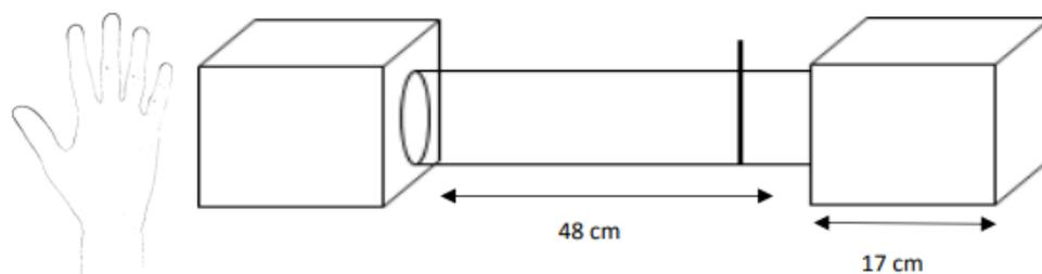
**Figure S5. Experimental set-up for behavioural bioassay.** A schematic of short range behavioural assay. Mosquitoes were released into a mesh holding cage that was 17cm x 17cm x 17cm. A tube 12cm in diameter and 48cm in length connected this cage to another one of the same dimensions. A gate prevented movement from one cage through to the other until the assay was ready to begin.
