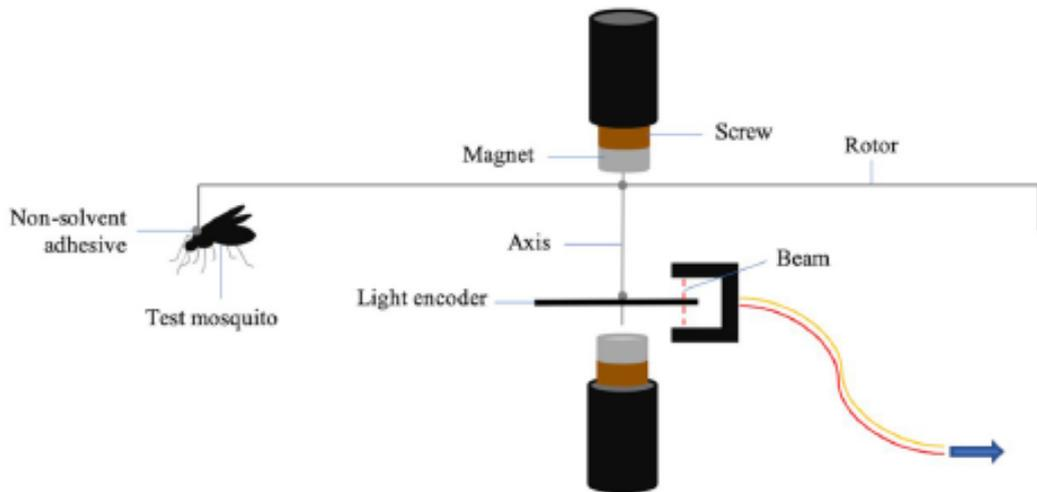
Figure 17. The set-up of a flight mill used during testing in this study, including rotor. Mosquitoes fly around a radius measuring 4cm, causing the light encoder to periodically break a laser beam with measures distance. 1 rotation = 25.13cm. (Image provided by A. Somerville).
