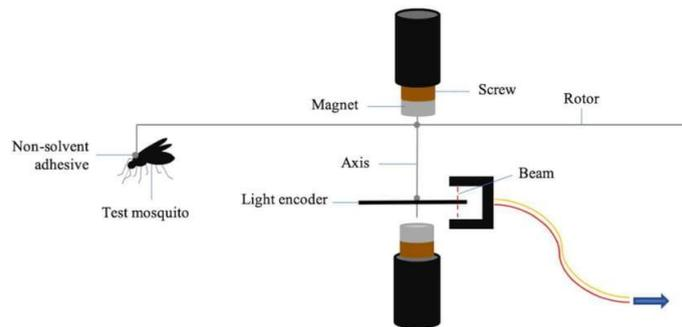
**Figure 3.** The set-up of a flight mill used during testing in this study, including rotor. Mosquitoes fly around a radius measuring 4 cm, causing the light encoder to periodically break a laser beam which measures distance. 1 rotation = 25.13 cm. Image provided by A. Somerville.
