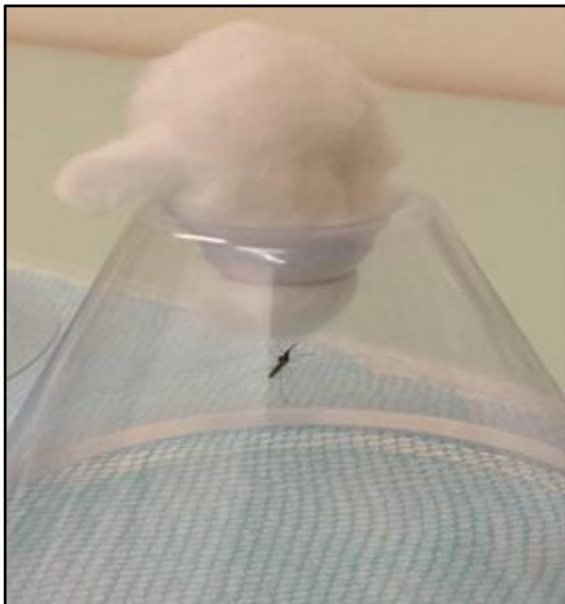
Figure 1.5 Example of WHO cone bioassay. Note that the mosquito is avoiding contact with the insecticidal net by resting on the untreated cotton wool.
