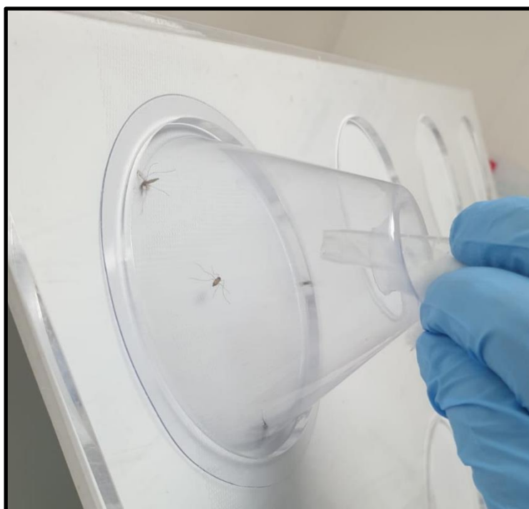
Figure 2.2 Example of WHO cone bioassay. Testing backboard is angled at 45 degrees to discourage avoidance from the net.
