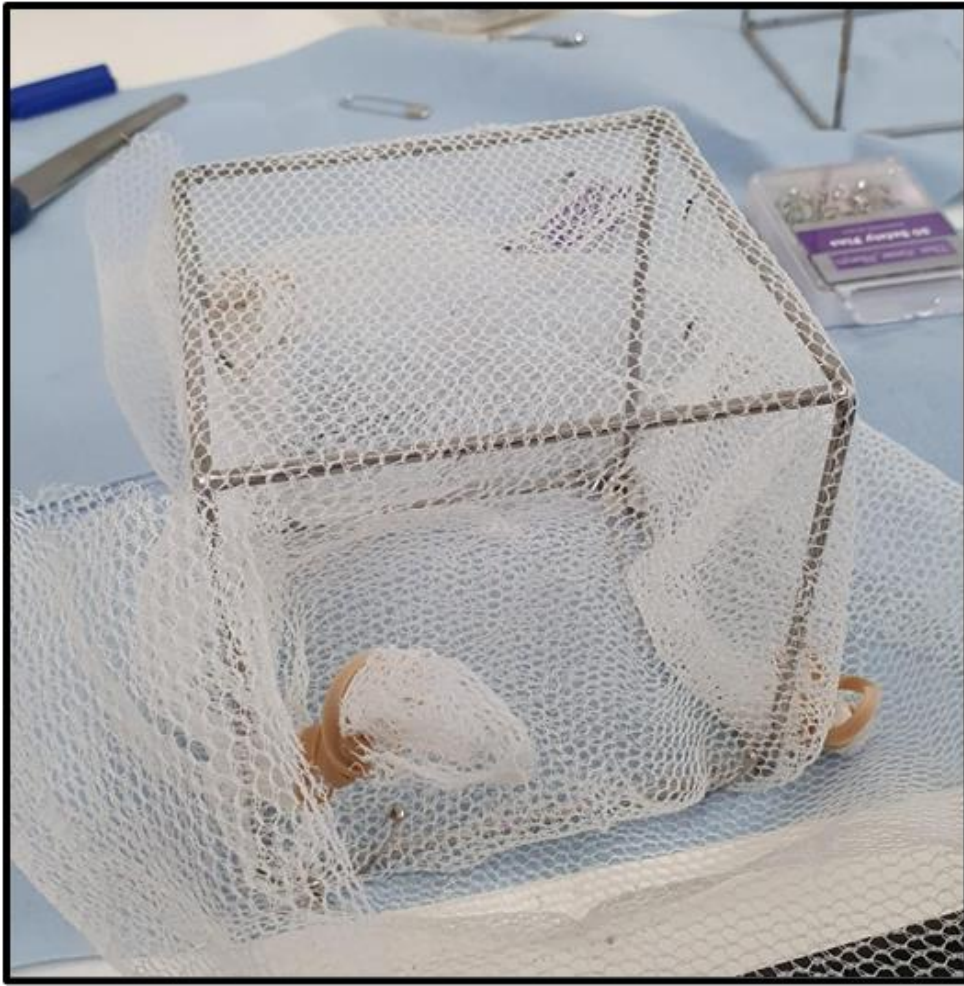
Figure 2.3 Image of cube variant of WHO wireball assay in use. Image shows netting material wrapped around the metal cube frame and secured in place with elastic bands. Mosquitoes are released into the cube by a 'sleeve' of excess material.
