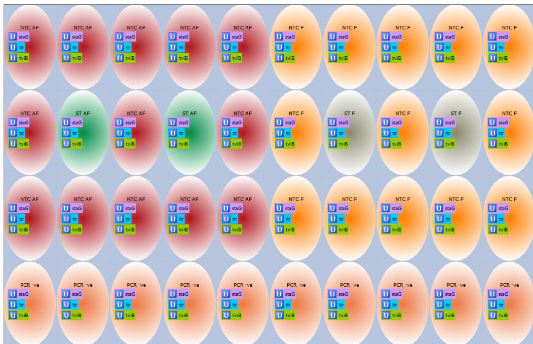
Figure 4.10: Layout of the samples used to assess contamination during extraction with the QiaVAC and DNeasy 96 well kits, for both extraction and the real time PCR assay. NTC AF: Non-template control with anti-foaming agent, ST AF: S. Typhi control with anti-foaming agent. NTC F and ST F: Non-template control and S. Typhi control without anti-foaming agent, respectively.
