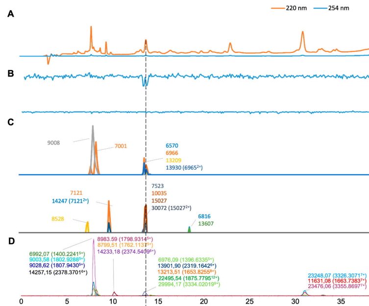
Figure 2. Integrated Bitis arietans venom results: superimposed results of LC-UV data, LC-(ESI)-MS data, and nanofractionation MALDI-MS data plotted chromatographically and nanofractionation
