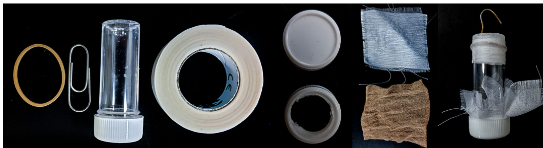
Figure 1. Components used to construct small sugar feeders for use in resource-limited insectaries. From left to right: elastic band, paperclip, 8 mL bijou, medical tape, bijou lid with drilled hole, various materials, assembled sugar feeder.
