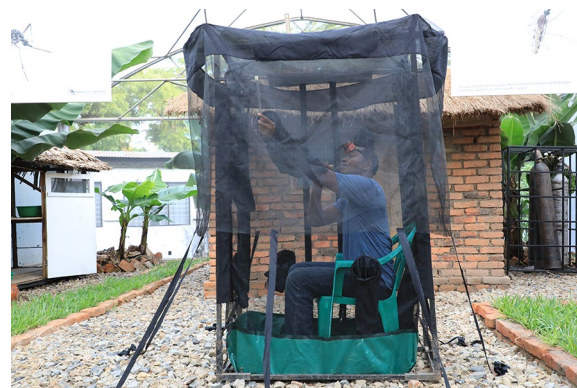
Fig. 2 Miniaturized double net trap (DN-Mini) for sampling host-seeking mosquitoes indoors and outdoors. Picture was adapted from Limwagu et al. [10]
