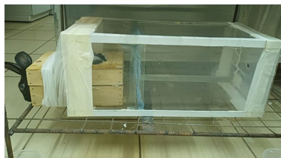
Fig. 2 A Tunnel assay set up in the laboratory to assess mosquito mortality and blood feeding success with dual active LLINs
